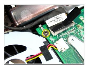
Loosen the screw that secures the low-voltage differential signaling (LVDS) cable.
