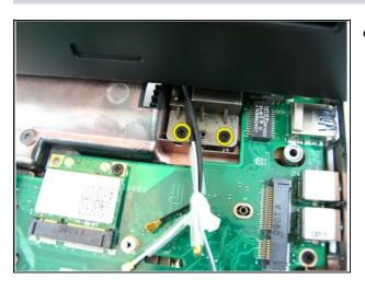
• Remove the screws that secure the right hinge.
