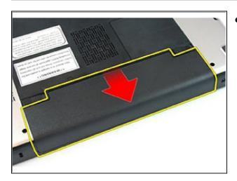
• Slide the battery and remove it from the computer.
