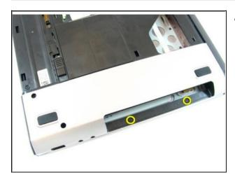
• Remove the screws in the optical drive compartment.
