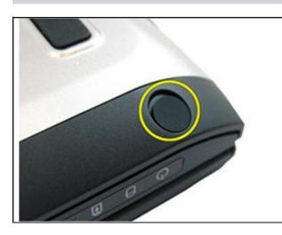
• Remove the rubber from the bottom base on the left side.
