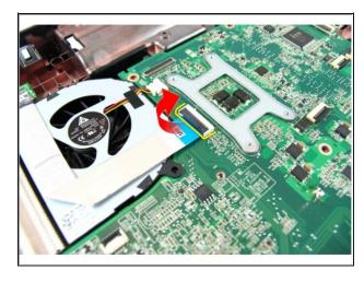
• Release the latch on the system board and then disconnect the VGA cable.
