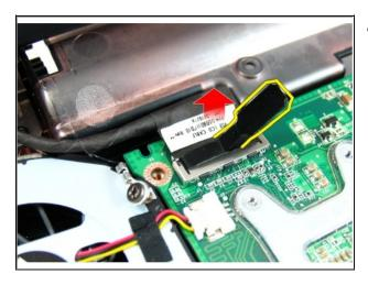
• Disconnect the LVDS cable from the system board.
