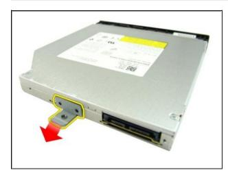
• Remove the optical drive bracket from the optical drive module.
