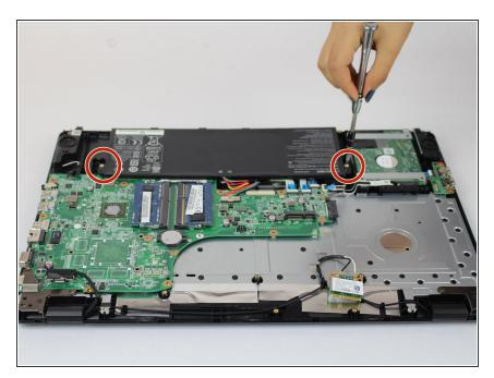
Remove the two 6mm Phillips #0 screws from the battery.
