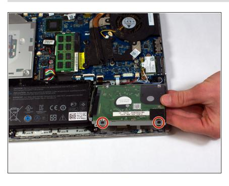
Remove the four additional 3.5mm screws using the Phillips #0 screwdriver.
