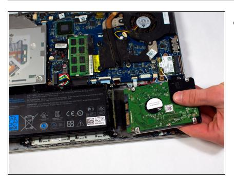
Carefully pull and remove the old hard drive.
