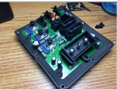
Carefully remove the 3 knobs and the 1 screw between the 2 10A fuses. then the plastic face should pop off
