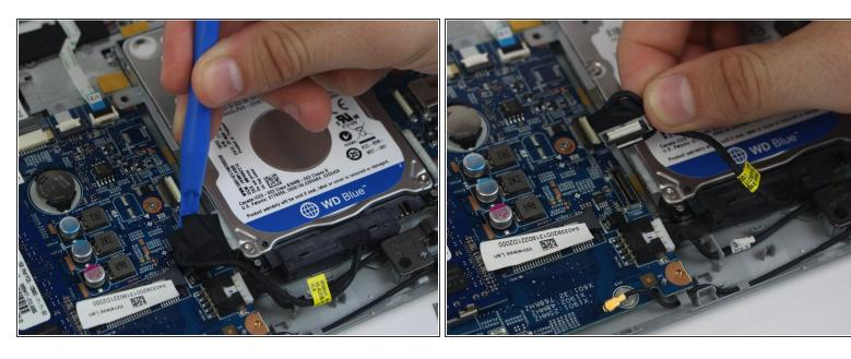
Disconnect the data connector from the motherboard using a plastic opening tool.
