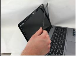
Using the metal spudger, pry off the edges of the screen's frame from the outside.
