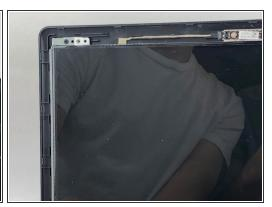
There should be four silver brackets holding the screen in place underneath. Unscrew the center
