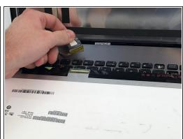
Place the monitor face down. Slowly remove the adhesive tape on the back of the monitor, and remove the connector that the tape is holding.
