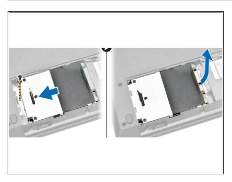
Loosen the screw securing the hard drive and lift the hard drive off the computer
