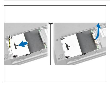
Remove the screw that secures the hard drive to the computer and slide the hard drive from the computer.
