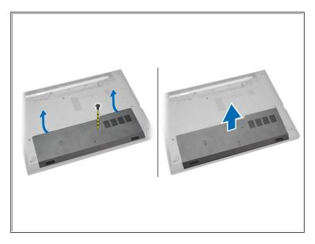
Loosen the screw and lift the access panel off the computer.
