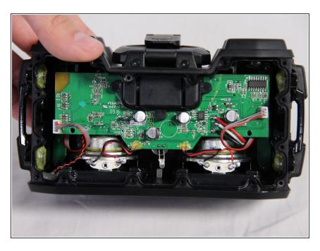
Carefully lift away the housing and replace the broken casing/component. Replace using the new casing.
