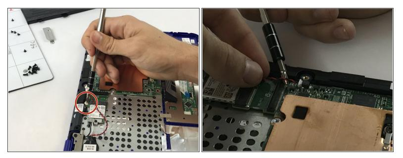
• Remove the 2mm screw that secures the motherboard and keyboard assembly.
