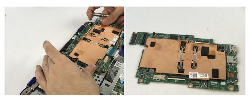
Lift the mother board off the palm rest and keyboard assembly.
