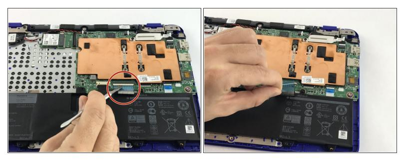
• Open the latches and disconnect the touch-pad cable and keyboard cable from the system board.
