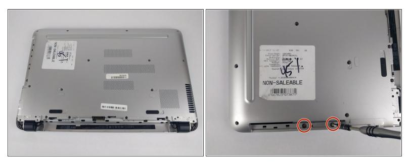
• With the CD drive removed, unscrew the two 2mm silver screws with a PH00.
