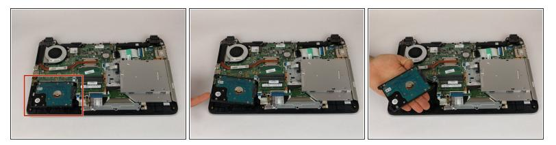
Locate the hard drive and lift up to give better access to the connector.
