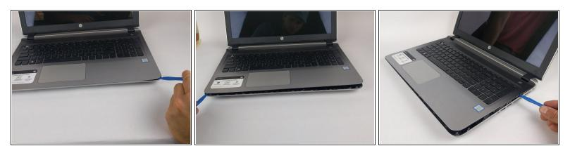
• Using a plastic opening tool, begin to pry edge of case away from the laptop. Work around the edges until all sides, except back, are open.
