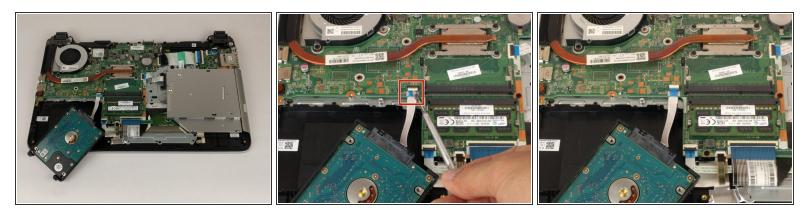
• Using a plastic opening tool or spudger, pry open the white tab to release connector.
