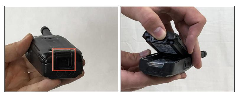
• Push in the release button and pull up on the battery to remove.
