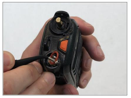
• Remove the orange o-ring around volume knob using tweezers.
