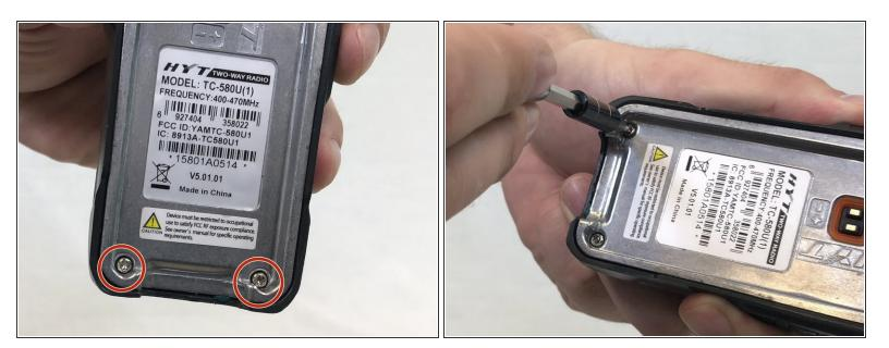
• Remove the two 15mm T8 Torx screws from the base of the battery cavity.
