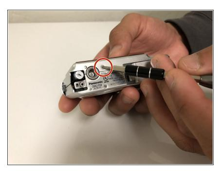
Remove the screw located on the base of the camera.
