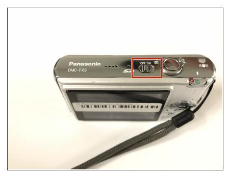
Power off your device by locating the on/off switch on top of camera.
