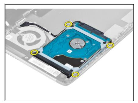
Remove the screws that secure the hard drive to the computer.
