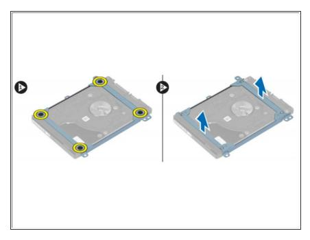
Remove the screws that secure the hard-drive bracket to the hard drive and remove the hard drive bracket from it.
