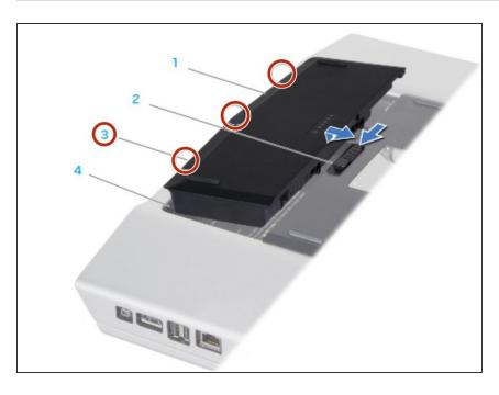
Align the battery pack tabs with the slots in the battery bay.
