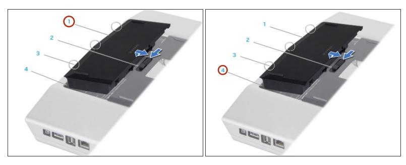
Slide the NEW battery pack into the battery bay until the battery pack clicks into place.
