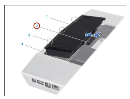
Slide the battery latch to the unlock position as shown.
