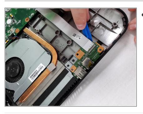
Use plastic pry tool to lift up on headphone jack assembly
