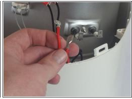
Disconnect the red wires from the inner liner.
