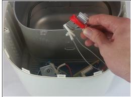
• Use a spudger to push out the connector found on the inner lining.
