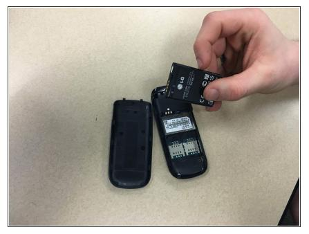
• Gently remove the battery from the device.
