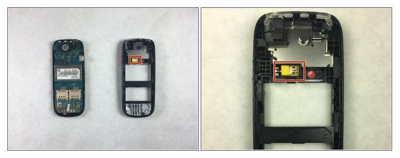
• After separating the two plastic halves of the phone, take the plastic that does not have the motherboard attached to it. The plastic has a small yellow component with a lob-sided magnet within it. This is the vibrator of the phone, pull this piece out with your hand. This piece is free floating and will simply drop out.
