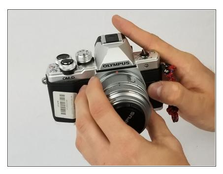
While holding down the button specified in step 1, begin turning the inner most ring, specified in step 2, counterclockwise until the camera lens becomes free from the camera body.
