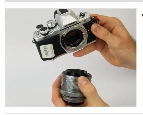
Once the lens is free from the camera body, pull the lens completely away from the body to make sure the lens is truly free.
