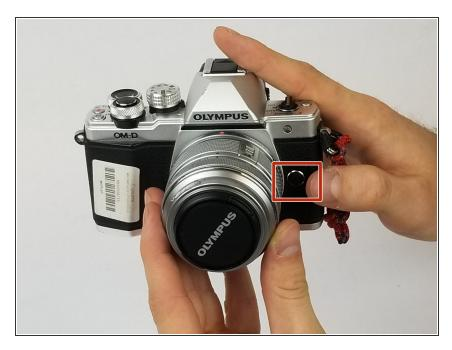
Press the black button located to the right of the camera lens when facing the front of the camera.
