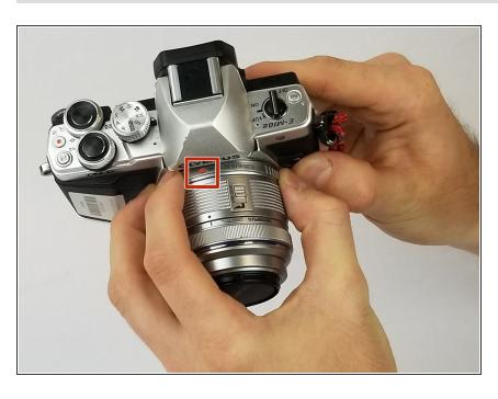
Grasp the innermost ring on the lens, closest to the camera body, which can be located by the small red dot. This is the only ring that should not turn, unless the button specified in the previous step is held down.
