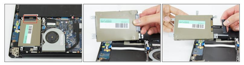
• Lift the hard drive up and remove the power supply cable connected to it.
