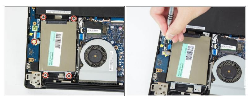
Using the JIS #0 Screwdriver, remove the five 3.0 mm screws that hold down the hard drive casing.
