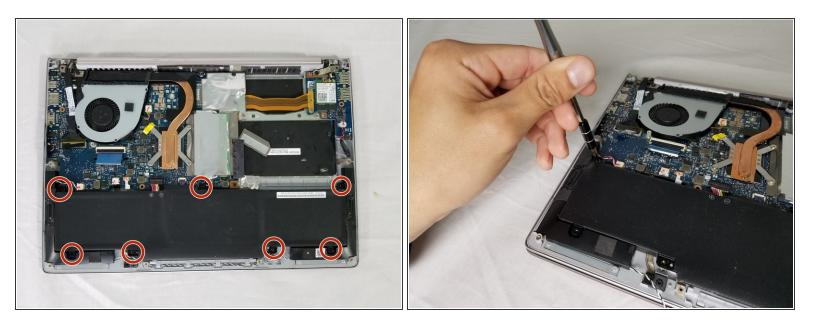
• Remove all seven 2 mm Phillips #00 screws from the battery.
