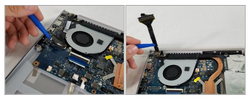
• Disconnect the display cable from the motherboard with a plastic opening tool.
