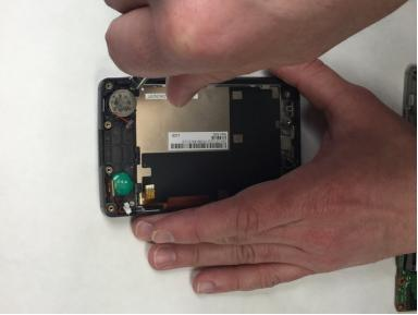
Remove the two 9.6 mm screws by the speaker and green battery with a JIS #0 screwdriver.
