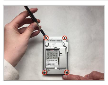
Remove the four 12.7mm screws under rubber feet with a JIS #0 screwdriver.
