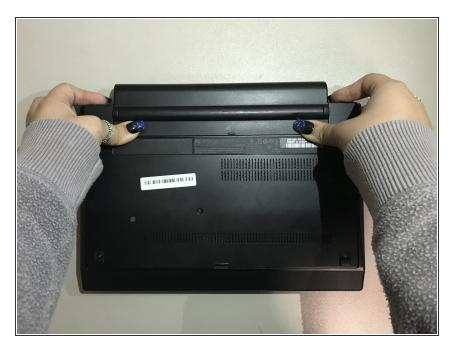
• Use your fingers to push both battery release tabs on the back of the computer.
