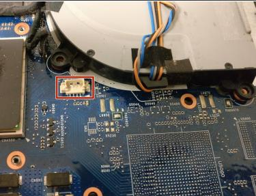
Gently disconnect the wire connecting the fan to the motherboard
