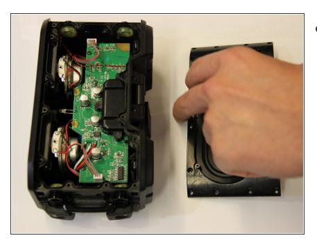
Carefully lift away the broken subwoofer plate of the device. Replace with functioning sub-woofer plate.
