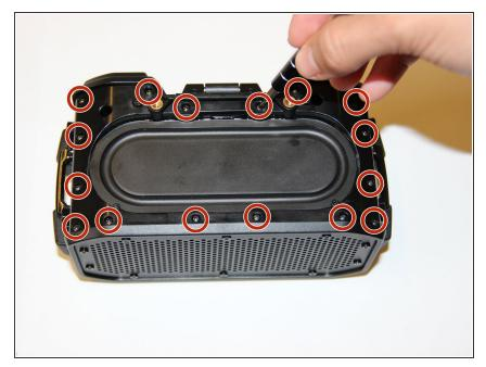
To remove the hard inner plastic casing, use a Phillips #00 head bit to remove the 16 small 9mm screws surrounding the subwoofer on the top side of the device.
