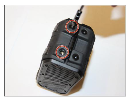
To remove the outer rubber casing use a 3mm Hex bit to remove the 4 large 12mm Hex screws on both sides, found on the bottom part of the device.
