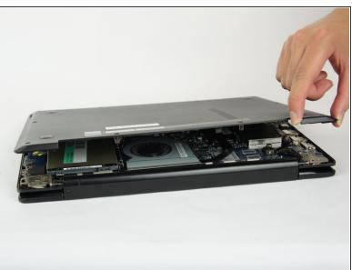
Insert the flat edge of the opening tool in between the back casing to remove the back casing.
