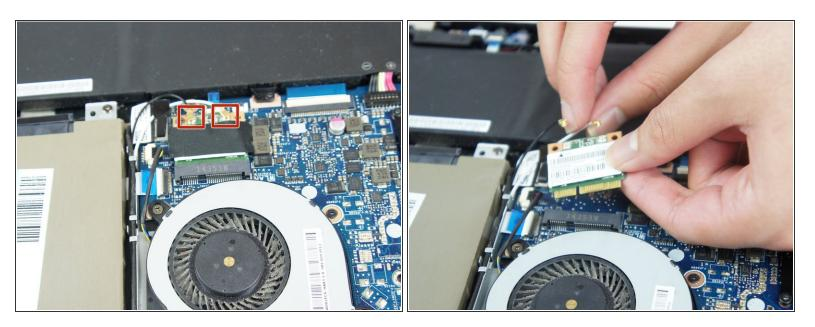
Disconnect the black and white wires that provide power and data transfer to the Wi-Fi chip.
