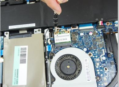
• Use a JIS #0 Screwdriver to remove the one 3.0 mm screw.
