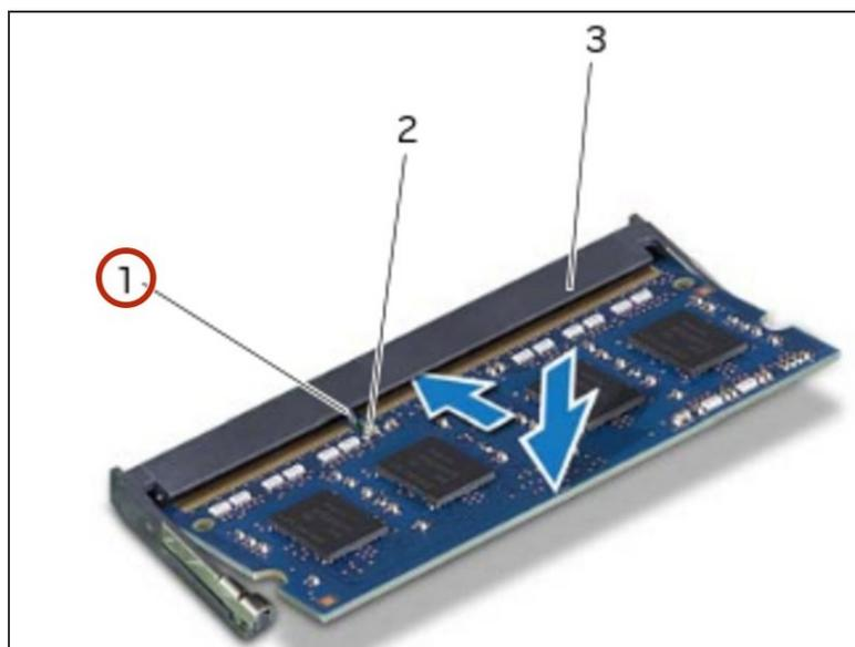
**i** NOTE: If you need to install memory modules in two connectors, install a memory module in the lower connector before you install a memory module in the upper connector.
