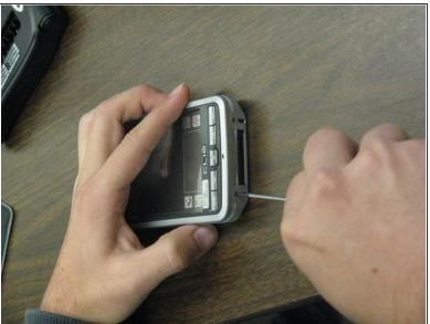
● 1. Unscrew the six screws on device. (2 screws on left side, 2 on right side, 2 on bottom)
