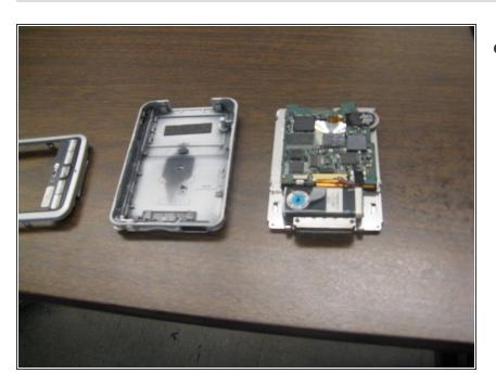
3. Pull the screen out of the back case with iPod opening tool. The device should now be in three different parts.
