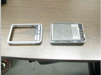
2. With an iPod opening tool, lift the front cover (face plate) from the device.
