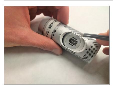
Insert the tweezers into the crevice of the ball and socket joint, and prop up the tabs to remove the white ring from the body.
