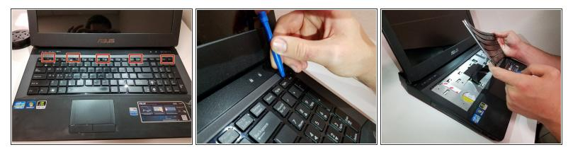
Insert a spudger, or plastic opening tool, into these five slots and pry upwards to pop up the keyboard.
