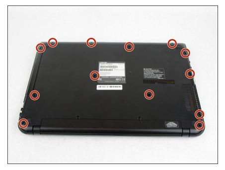
Remove the remaining thirteen 7 mm Phillips screws holding the back cover using the PH1 bit and Magnetic Driver.
