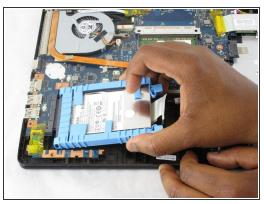
Using the ribbon beneath the hard drive lift it upwards and pull the hard drive out.
