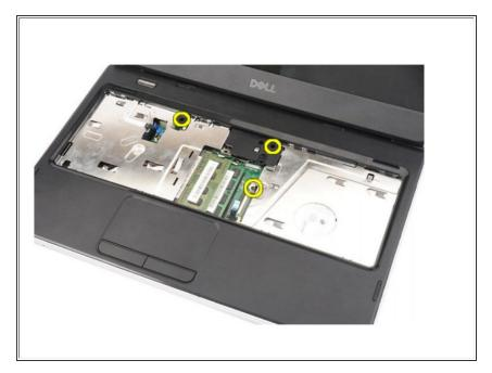
Remove the screws that secure the palm rest to the computer.
