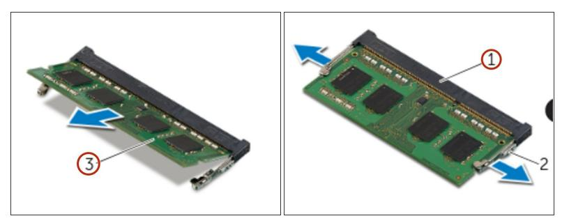
Remove the memory module from the memory-module connector.
