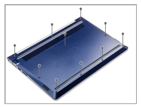
Remove the screws that secure the back cover to the computer
