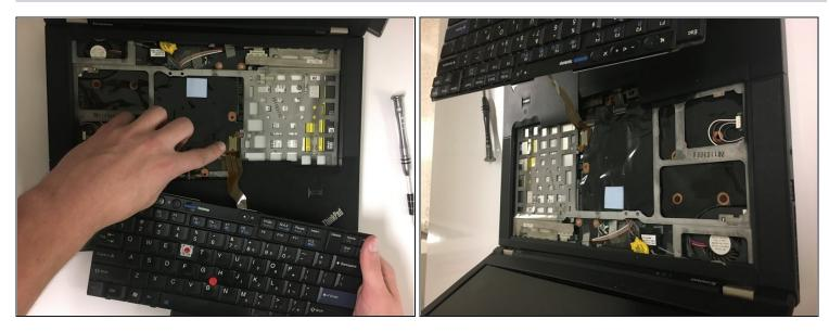
• Slide the keyboard out of the way until you can see what's underneath it.
