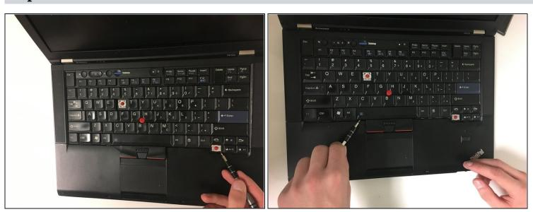
Wedge the flat end of a spudger, or plastic opening tool, under the end of the keyboard and pry up.
