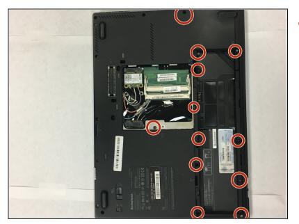
• Remove the twelve Phillips #0 screws from the back panel.
