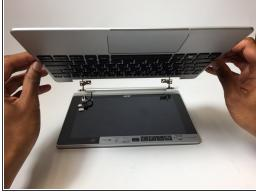
Carefully pull up on the keyboard section using your hands to remove it from the screen section.
