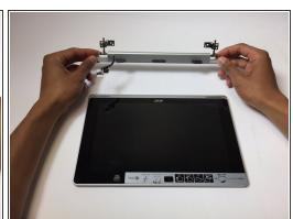
Pull the docking connector off of the screen section.
