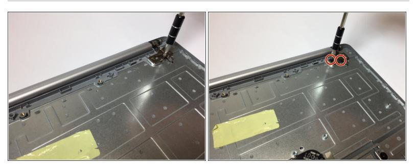
Remove the 2, 4.25 mm screws on the right hand tab that are securing the dock in place.
