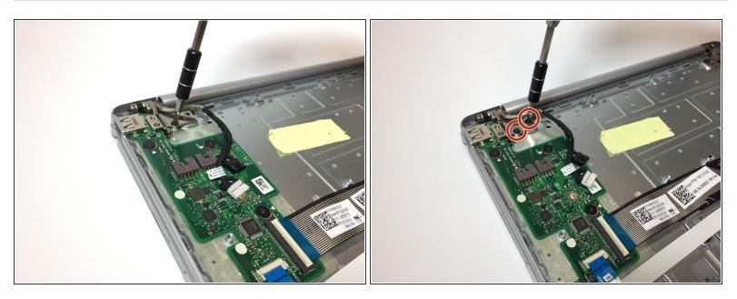
Remove the 2, 4.25 mm screws on the left hand tab that are securing the dock in place.
