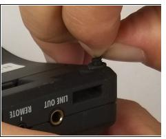
• With device facedown, lift the four rubber feet from the device using tweezers or fingernails.
