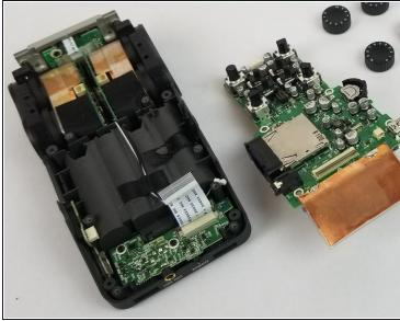
• Gently lift the motherboard from the base of the device and set aside.
