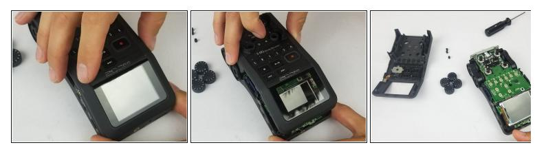
• With the bottom of the device on a table, lift the top of the device and gently place it aside.
