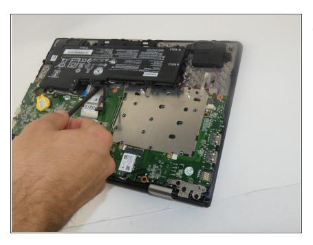
Lift the battery with a spudger and remove.
