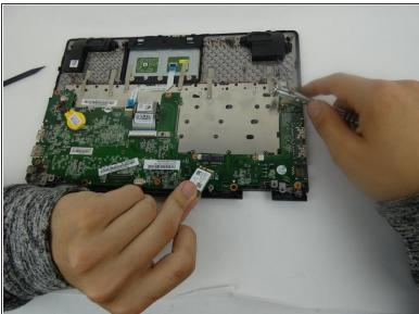
Remove the Wi-Fi card from the motherboard socket.
