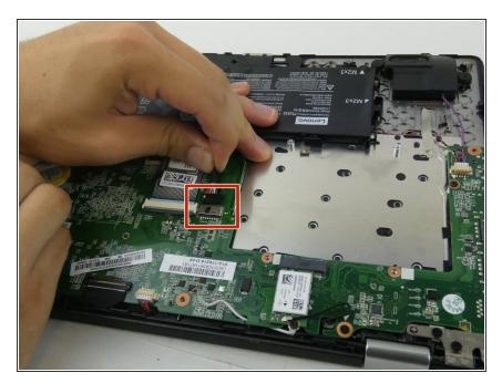
Remove the connector attaching the battery to the motherboard.
