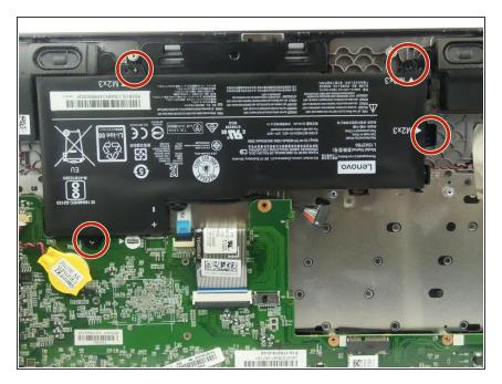
Remove the four 4mm screws on the battery.
