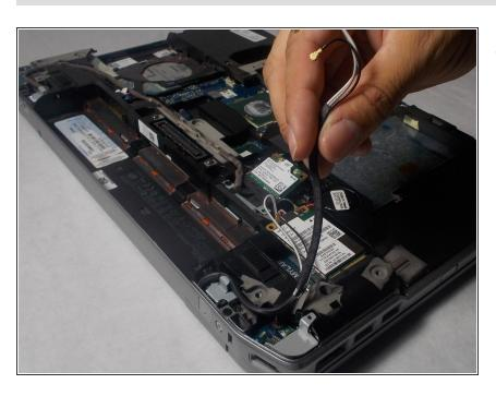
Lift the wiring harness out of the way.
