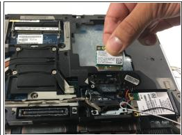
• The card will lift up, remove the card by pulling the lifted edge away from you.
