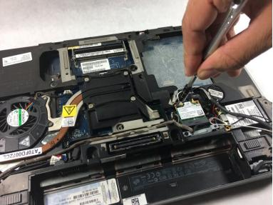
• Using the screwdriver, remove two 4mm JIS #0 screws.
