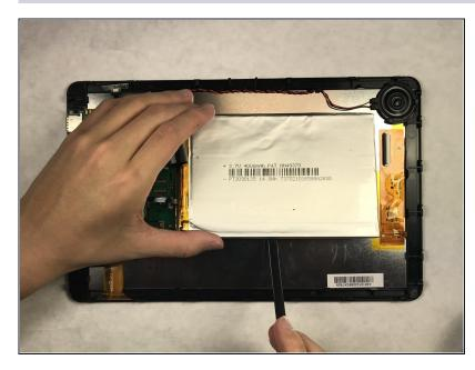
• Use nylon spudger tool or <u>plastic card</u> to separate battery from the case.
