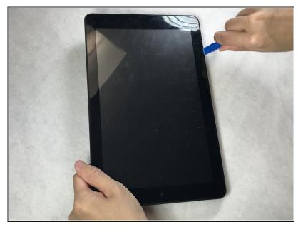
• Insert plastic opening tool and slide it around the edges until the cover starts to pop off. It may be necessary to go over each side multiple times in order to pop the cover off.
