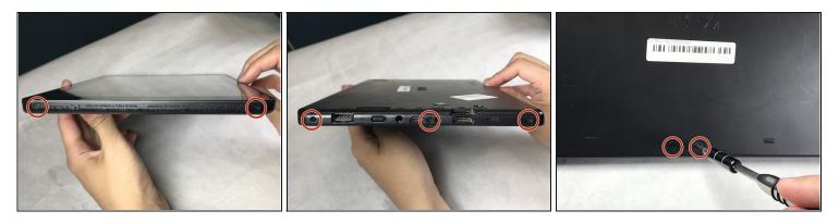
• Remove nine 4.8mm screws around the case with a JIS #00 screwdriver.
