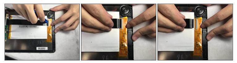
• Disconnect the thick black band (bus) using a plastic opening tool or fingernail.
