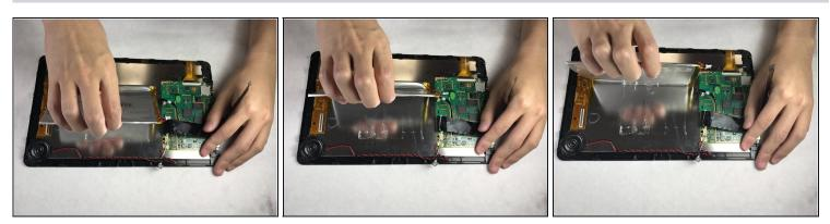
• Carefully peel off the battery.
