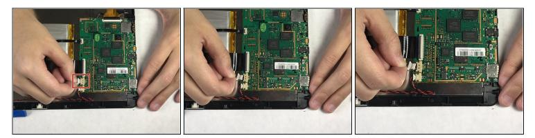
• Disconnect battery cable from the motherboard.
