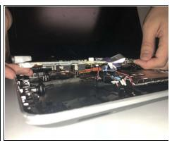
• Use the flat end of a spudger to disconnect all wires connected to the motherboard.
