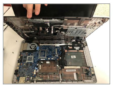
• Remove the panel by lifting it up.
