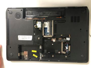
• Use the flat end of a spudger to pop off the antenna connectors.
