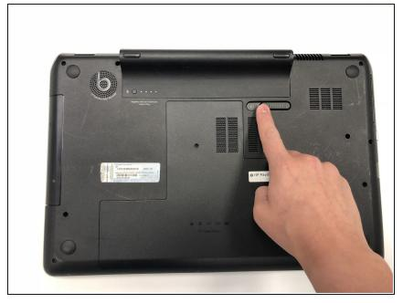
• Slide the battery release switch to the left.
