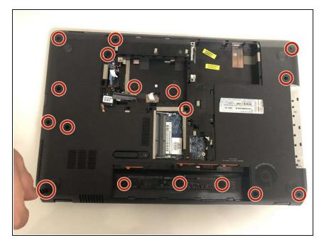
Remove the seventeen Phillips #00 screws securing the back panel to the laptop.
