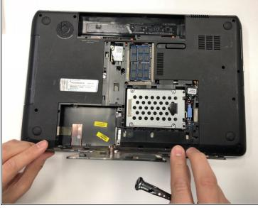
• Remove service hatch by sliding away from the computer and lifting up.
