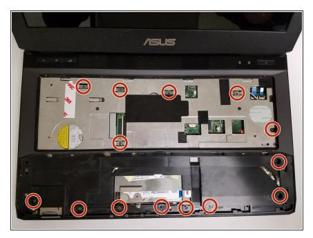
Remove the fourteen Phillips #0 screws.
