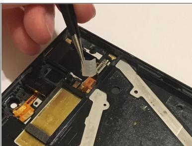
Use a pair of tweezers to remove the vibration boot that covers the module.
