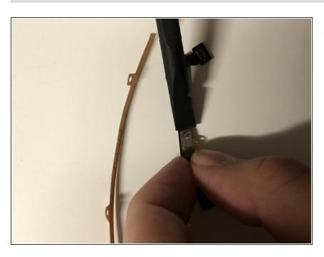
Repeat the previous step for the black jumper flex cable under the battery.
