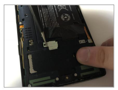
Use tweezers to remove the battery connector strap.
