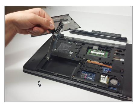
Finally, using the same tab, lift the hard drive out of the hard drive port.
