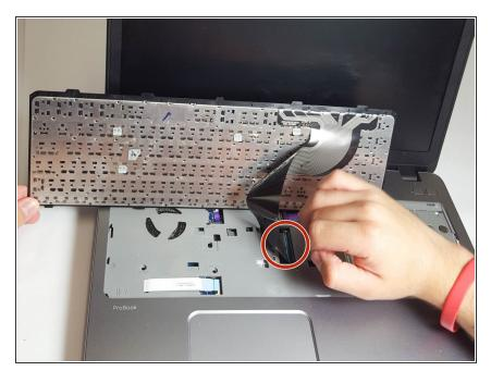
Disconnect the keyboard ribbon by carefully lifting the thin, black connector latch and separating the keyboard from the rest of the laptop.
