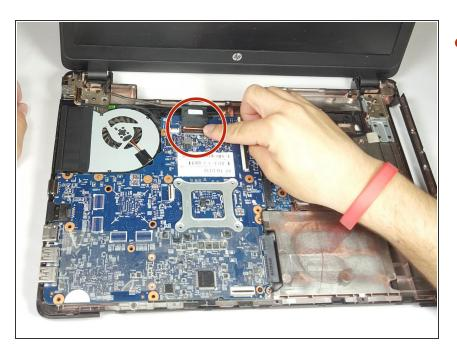
Disconnect the ribbon attached to the motherboard
