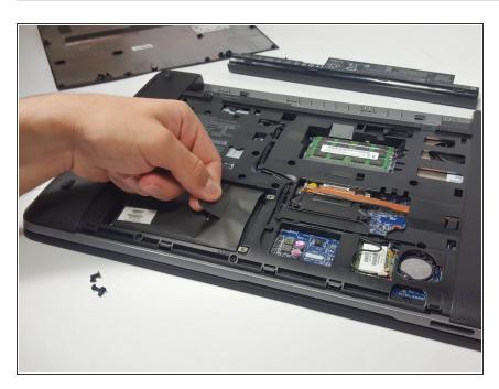
Pull the hard drive cover tab to the left in order to disconnect the hard drive from the computer.
