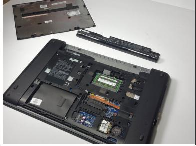
Using a Phillips #0 Screwdriver, remove the four Phillips 3 mm screws that secure the hard drive into the computer.
