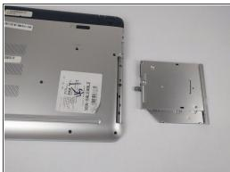
• Using your finger nail or a plastic opening tool, pull out the drive.
