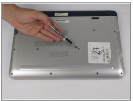
Locate the screw, will have a CD symbol next to it, and remove this 3.5 mm screw with a PH0 screw driver.
