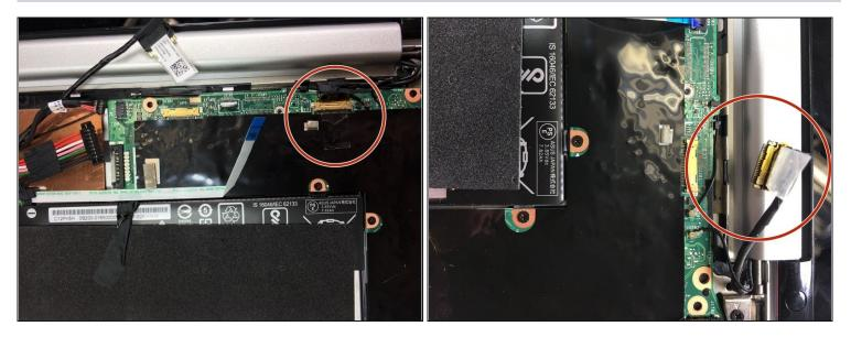
Disconnect the digitizer board cable from the motherboard using the pointed end of a plastic spudger.
