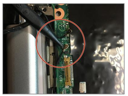
Disconnect the two WiFi antenna cables from the motherboard using the pointed end of a plastic spudger or simply by pulling the cables apart from the motherboard with your fingers.
