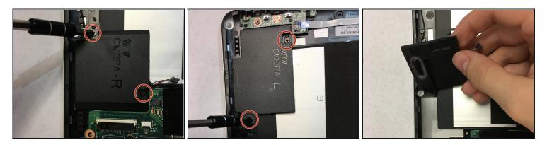
• Remove the four 4.2mm speaker screws, then remove the two speakers using a philips head screwdriver.
