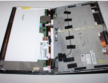
Carefully lift the screen up and flip it over onto the keyboard side as if you were turning the page of a book.
