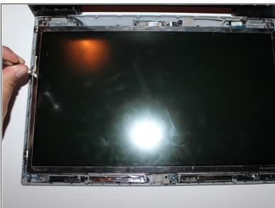
Remove the six 0.3mm Phillips #1 screws.
