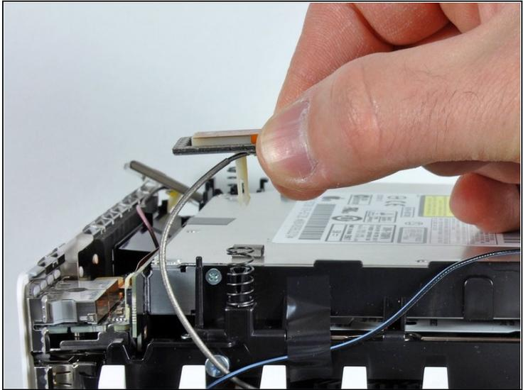
ⓘ The two Bluetooth antenna boards simply lift off the internal frame.
