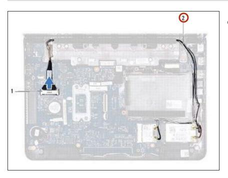
Connect the Mini-Card antenna cables to the Mini-Card(s).
