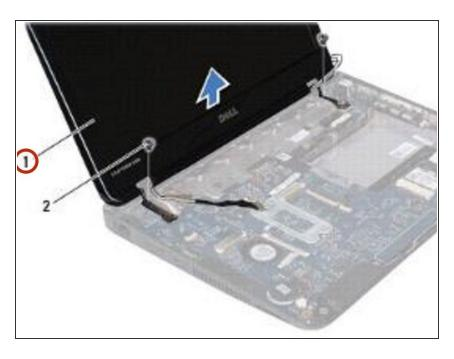
Lift and remove the display assembly off the computer base.
