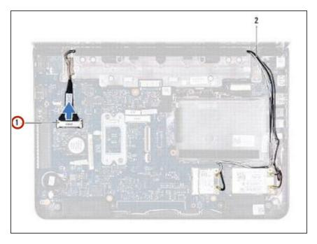
Disconnect the display cable from the system board connector.
