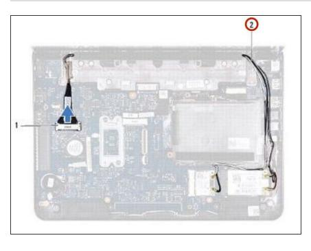
Route the Mini-Card antenna cables through the routing guides on the computer base.
