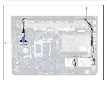
Make note of the cable routing and carefully dislodge the Mini-Card antenna cables from the routing guides.
