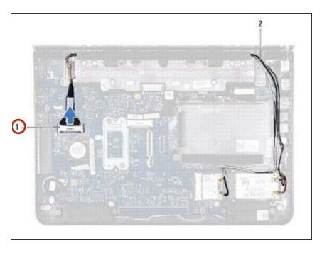
Connect the display cable to the system board connector.
