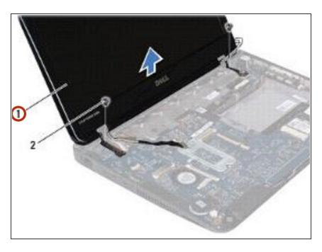
Place the **NEW** display assembly in position and replace the two screws (one on each side) that secure the
