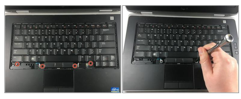
Using the screwdriver, remove four 3mm Phillips #0 screws from the keyboard.
