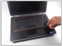
• Use the plastic opening tool to remove the bezel from around the keyboard.
