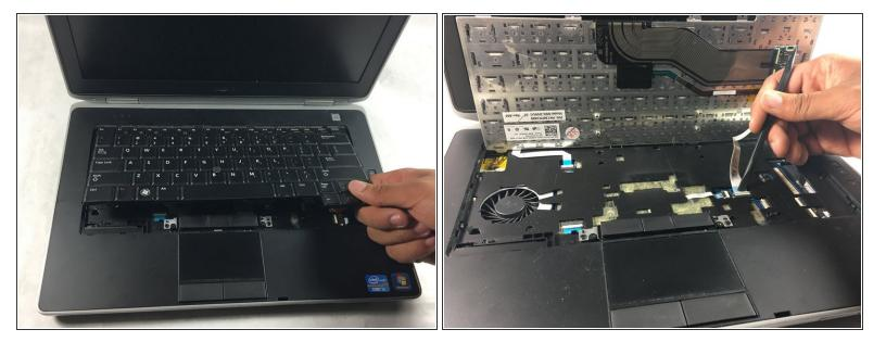
• Lift the keyboard and use the spudger to disconnect the keyboard cable.
