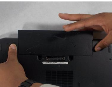
Push the tabs on the left and right of the battery out towards the edge of the case.
